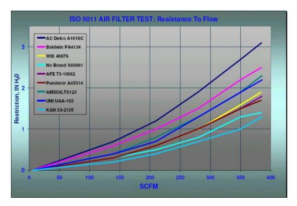
The Flow Restriction response curves for each filter have the same basic shape. However, note how the AC Filter, which passed the smallest amount of dirt and had the highest dirt capacity and efficiency, also had the highest relative restriction to flow. The less efficient filters correspondingly had less restriction to flow.
