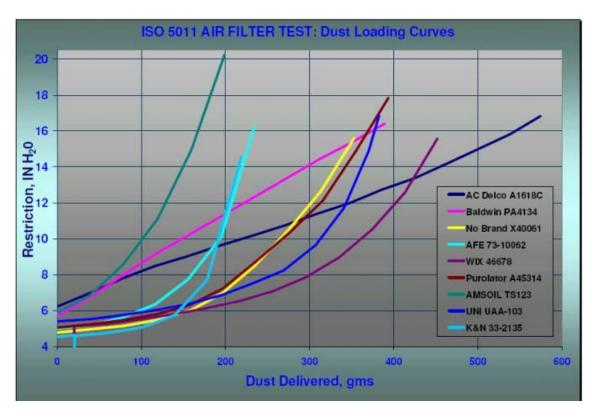
It's interesting to note the shape of these Dust Loading Curves. The AC and Baldwin filters each had near linear responses until reaching maximum restriction. Restriction for these filters increased at a constant rate versus the 9.8 gms/min dust feed rate.
