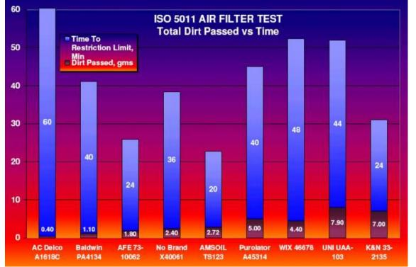
(Note: The Purolator was reported to have a seal malfunction during the test and passed more dirt than it would have with a good seal.)
